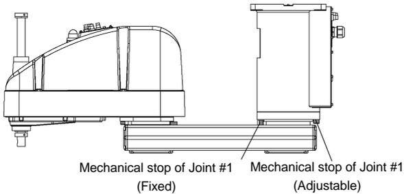
\* The different mechanical stop positions from Table Top Mounting are indicated for Wall Mounting and Ceiling Mounting.
