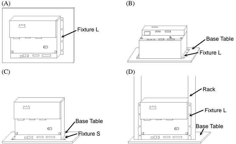
There are two types of fixtures. Mount the fixture to the Controller with the four attached screws.
