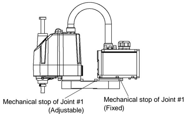
\* The different mechanical stop positions from Table Top mounting are indicated for Multiple mounting.
