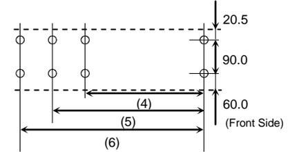
No screw hole processing is required for mounting direction (D).
