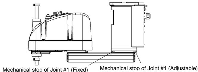
\* The different mechanical stop positions from Table Top mounting are indicated for Wall mounting and Ceiling mounting.
