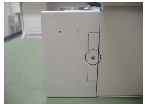
(5) Remove two screws on each cover.
