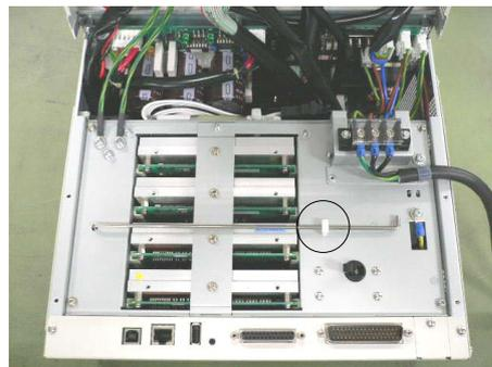
(7) Insert the top of the support bar into the support hole as shown without moving the base point.
