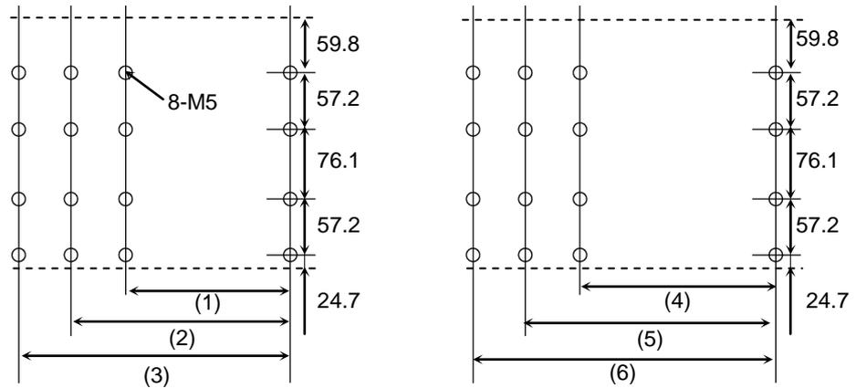
When mounting direction is (C) : Fixture S
