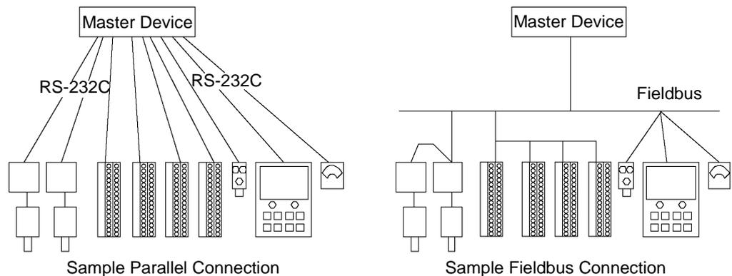
Fieldbus slave function can be added to the RC180 Controller. For each fieldbus on the controller, there is one board installed. You cannot use more than one fieldbus type on the same controller.
