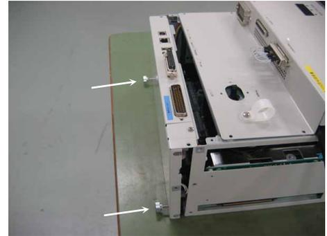
(3) Mount the screw on each side of the CPU board.
