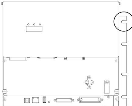
For Controller installation to the Controller box or the base table, process screw hole drilling as follows.
