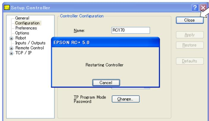
IP address configuration is completed and the Controller reboot dialog disappears.
