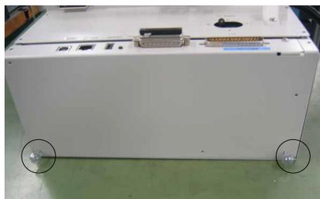
(9) Hold the thumb head screws and pull the CPU board unit straight out.
