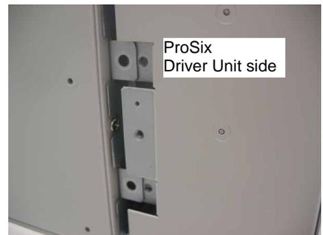
(5) Secure the ProSix Driver Unit with two screws on the top and bottom.
