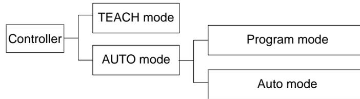
**TEACH mode** This mode enables point data teaching and checking close to the Robot using the Teach Pendant.
