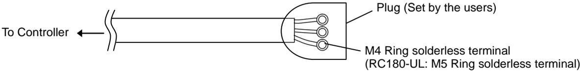
The AC plug in not attached to the AC power cable delivered at shipment. Refer to the wire connection specification and attach a proper plug to the cable that is suitable for the factory power supply. (A plug is prepared as option.)
