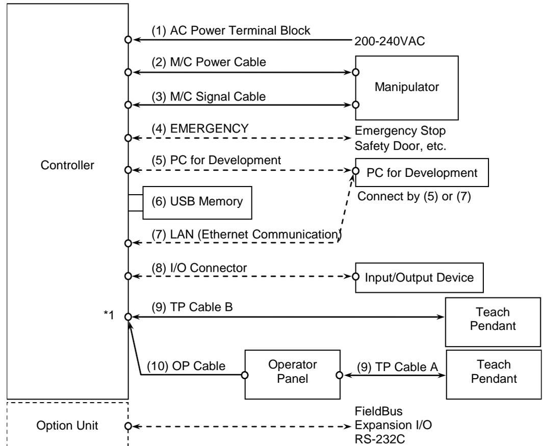
\*1 For this connection, only one of the connectors (9) TP cable B or (10) OP cable is connectable to the TP/OP port.
