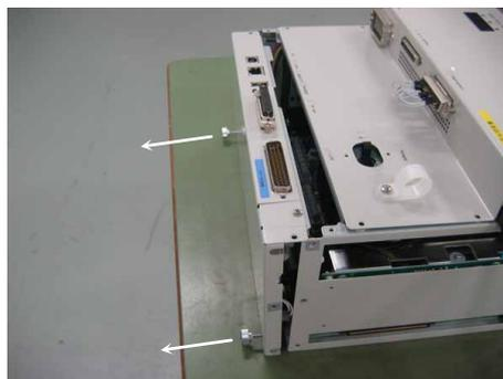
(10) Disconnect the four connectors connected to the CPU board.
