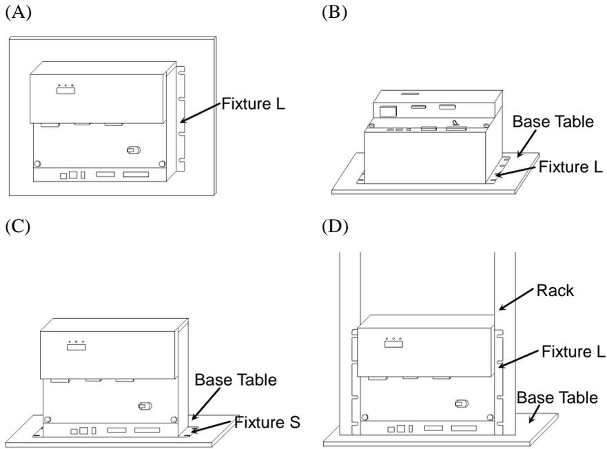
There are two types of fixtures. Mount the fixture to the Controller with the four attached screws.
