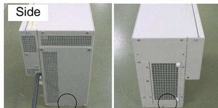
(8) Install the two thumb head screws removed in step (3) in the CPU board unit.
