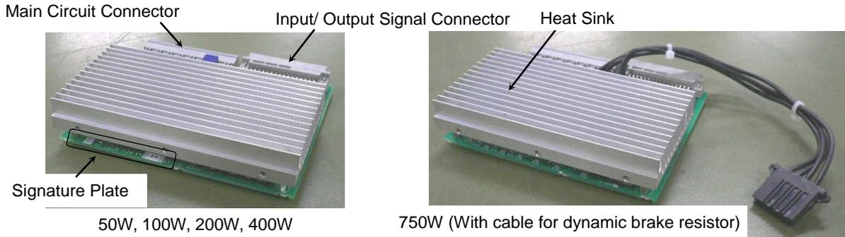
The wattage of the motor driver can be determined by the type code indicated on the signature plate. The wattage of the installed motor driver corresponds with the wattage of the driving motor.
