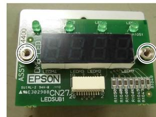
DMB-LED Board Installation (RC700DU-A)
