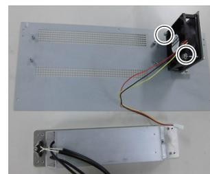
Regenerative Fan(1) Fix the new fan to the fan fixing plate. (Mounting screw ×2)
