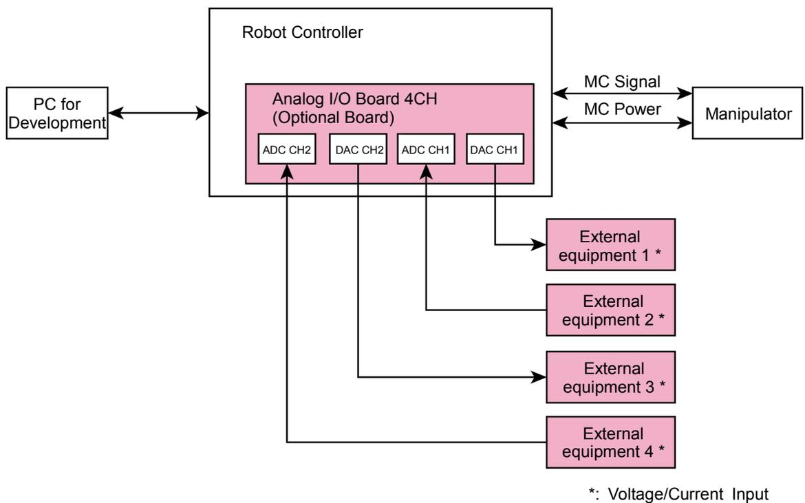
Overview of Analog I/O Board Circuit
