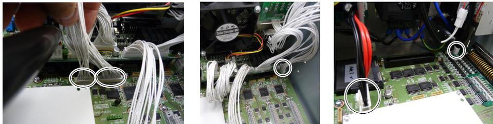
RC700-A: Connect the twelve connectors to the DMB.
