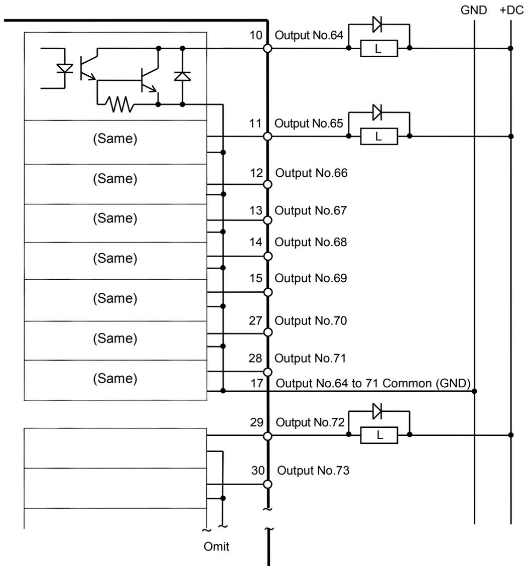
Typical Output Circuit Application 2: Source Type
