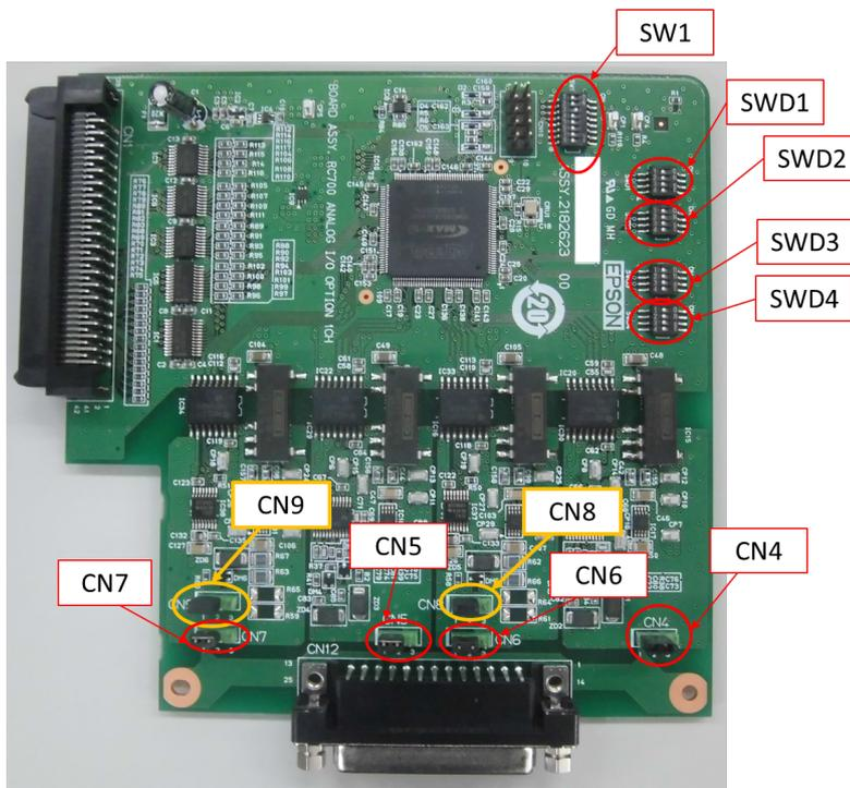
**Configuration of Switch and Jumper**
