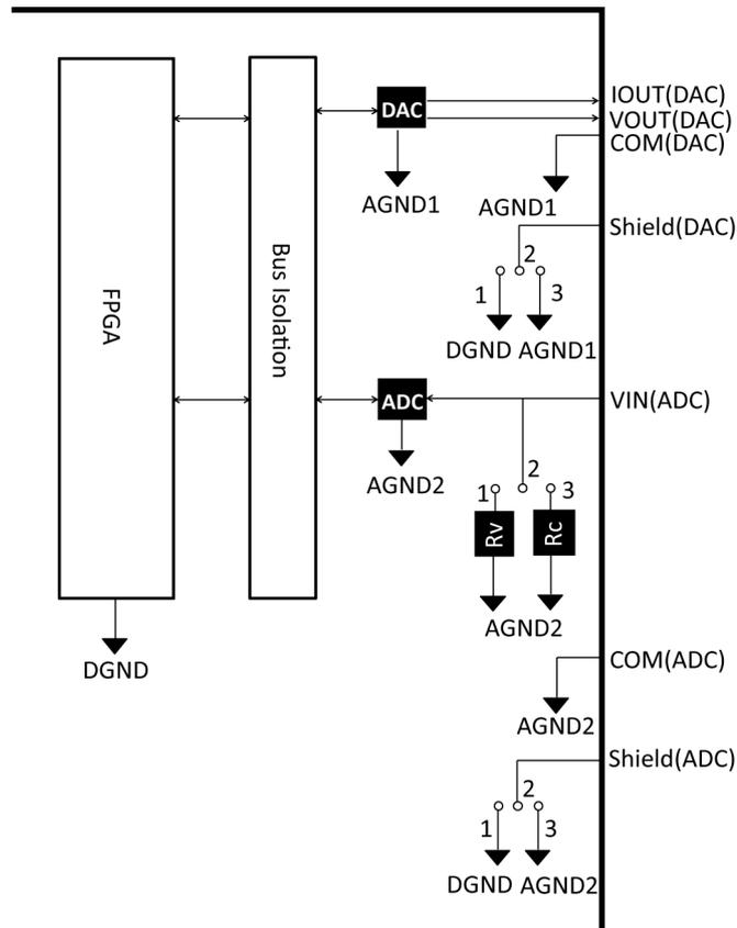
Rv: Voltage Input Terminating Resistance (100kΩ),
