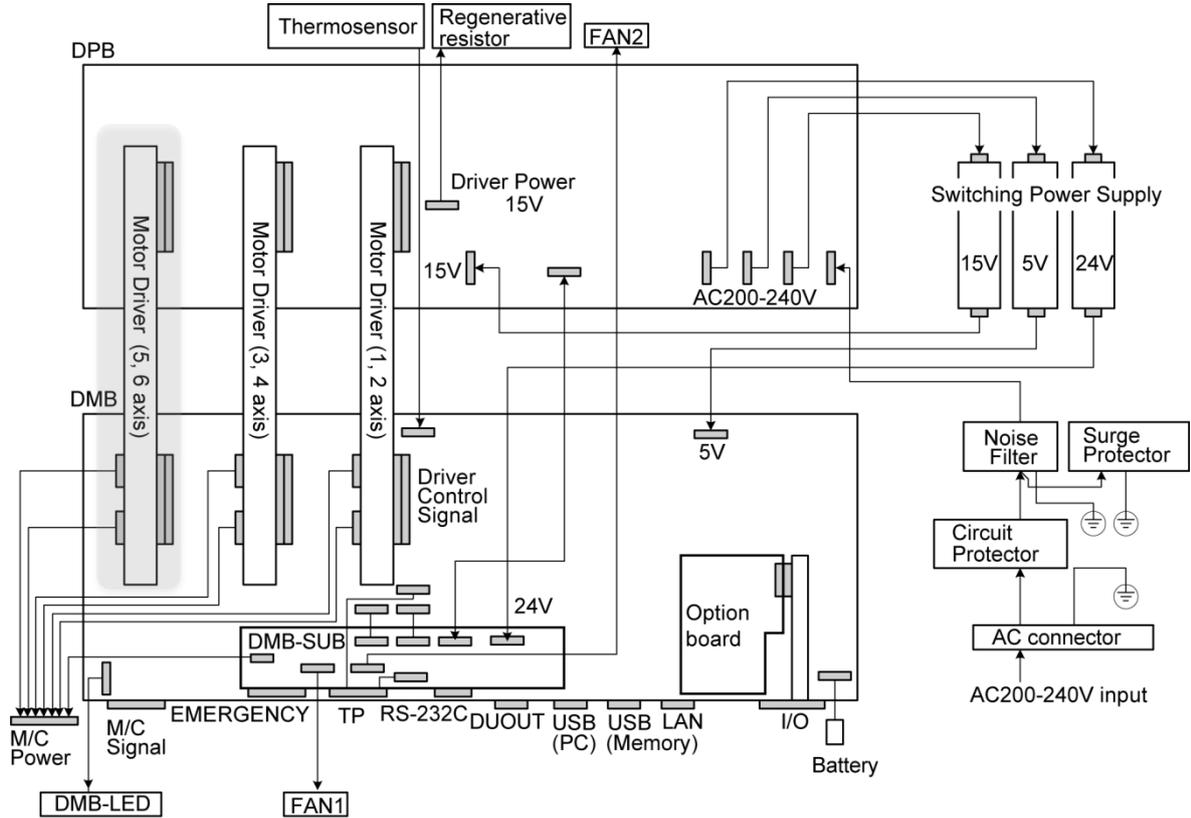
(Motor Driver (5, 6 axis) is not supplied for G1, G3, G6, G10, G20, RS and X5.)
