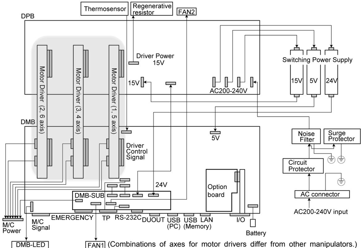
(Combinations of axes for motor drivers differ from other manipulators.)
