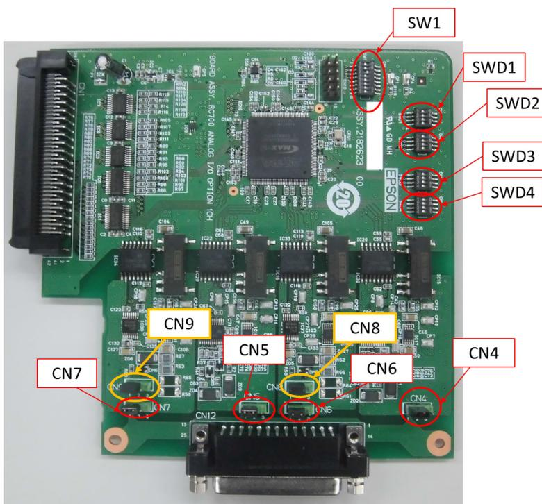
**Configuration of Switch and Jumper**
