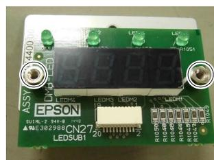
DMB-LED Board Installation (RC700-A)
