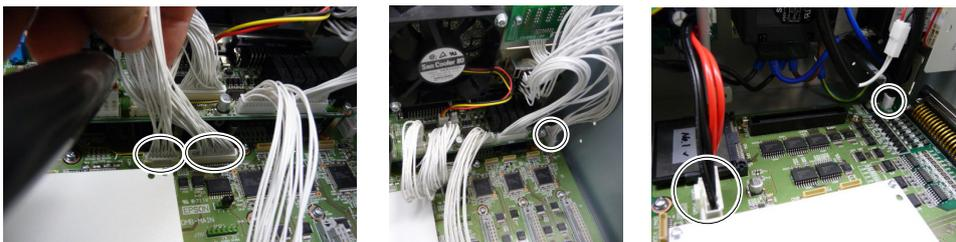
RC700-A: Remove the twelve connectors from the DMB.
