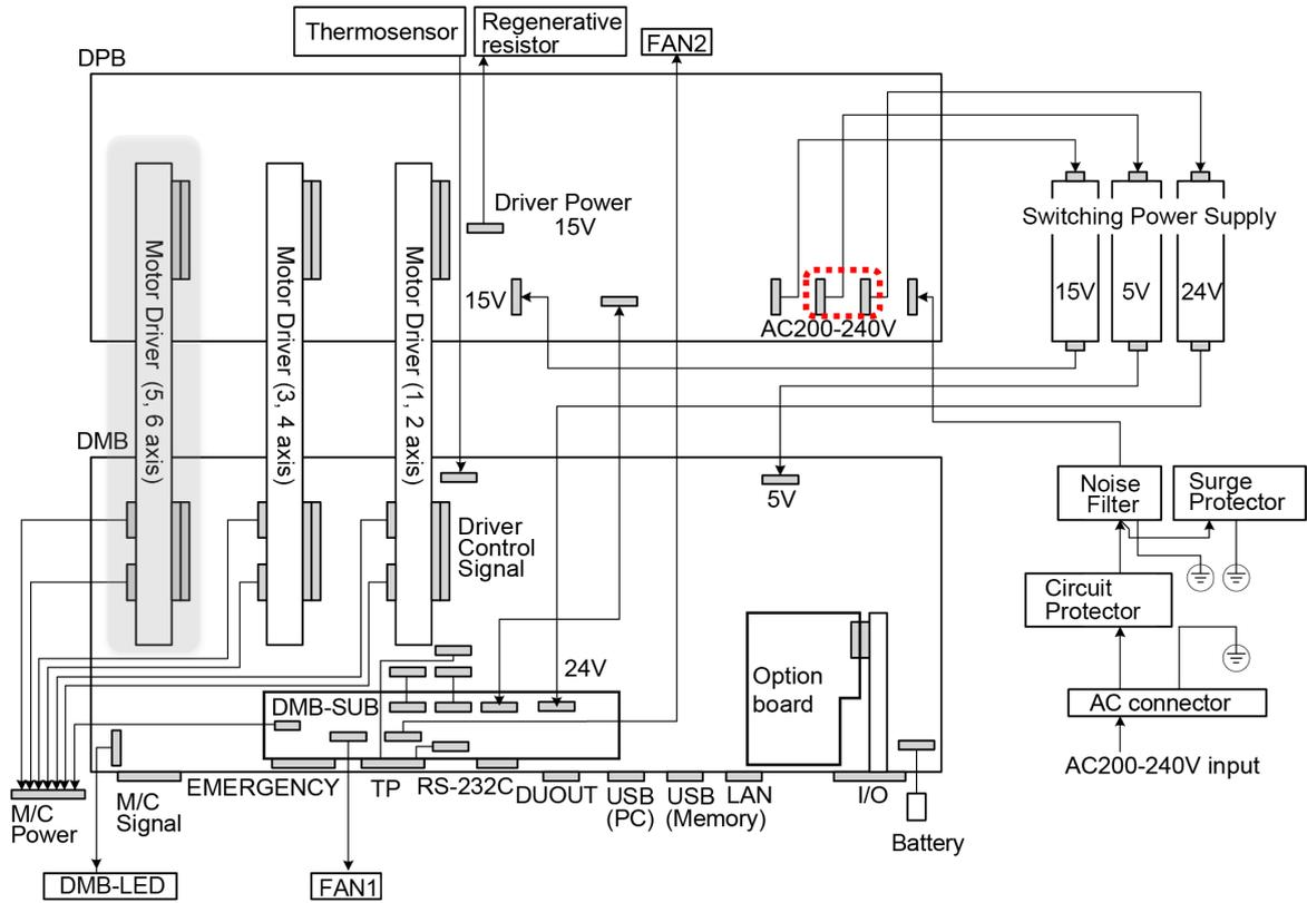
(Motor Driver (5, 6 axis) is not supplied for G1, G3, G6, G10, G20,RS and X5.)
