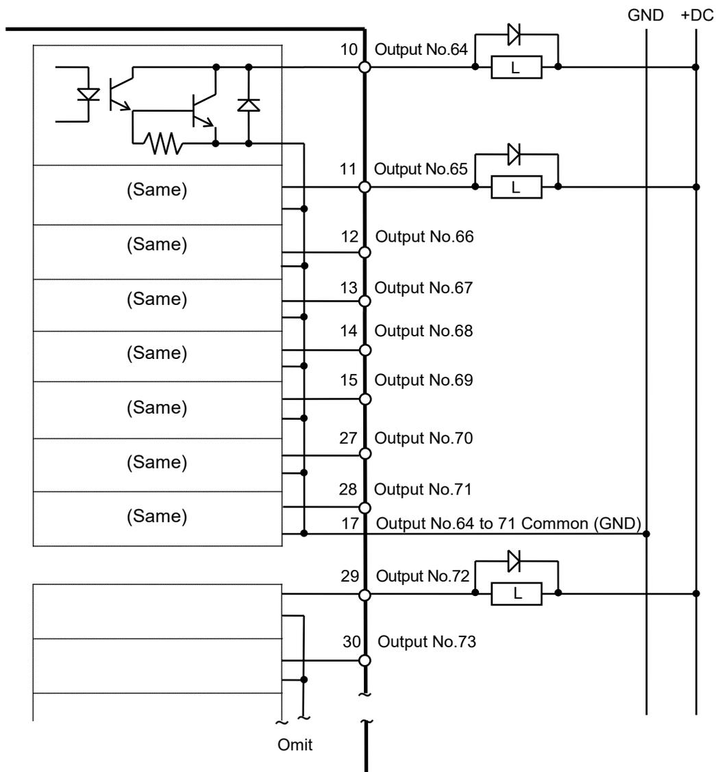
Typical Output Circuit Application 2: Source Type
