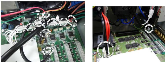
(10) Remove the DMB mounting screws (×14).
