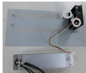
Regenerative Fan(1) Fix the new fan to the fan fixing plate. (Mounting screw ×2)
