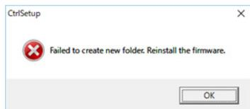
When the message is displayed, re-install the firmware.
