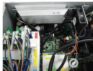
(6) Remove the regenerative module connector from the DMB.
