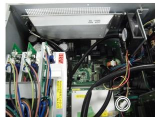
(6) Remove the regenerative module connector from the DMB.
