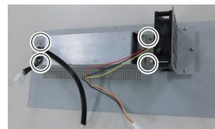
(10) Remove the fan from the fan fixing plate.
