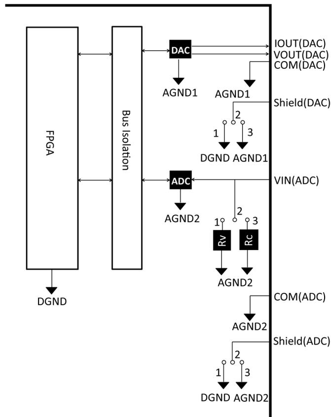
Rv: Voltage Input Terminating Resistance (100kΩ),
