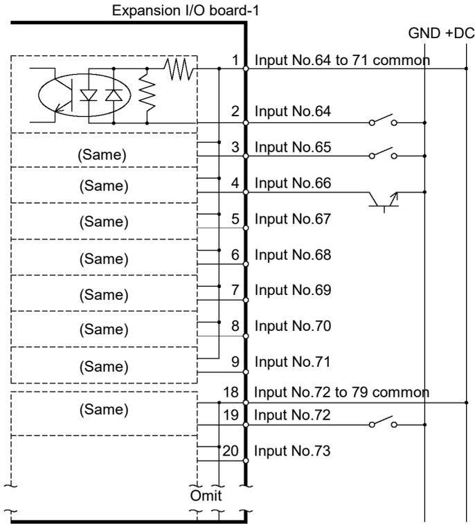
Protected Expansion I/O Board Typical Input Circuit Application 2
