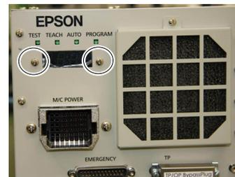
(4) Remove the LED/7 segment board from the Controller.
