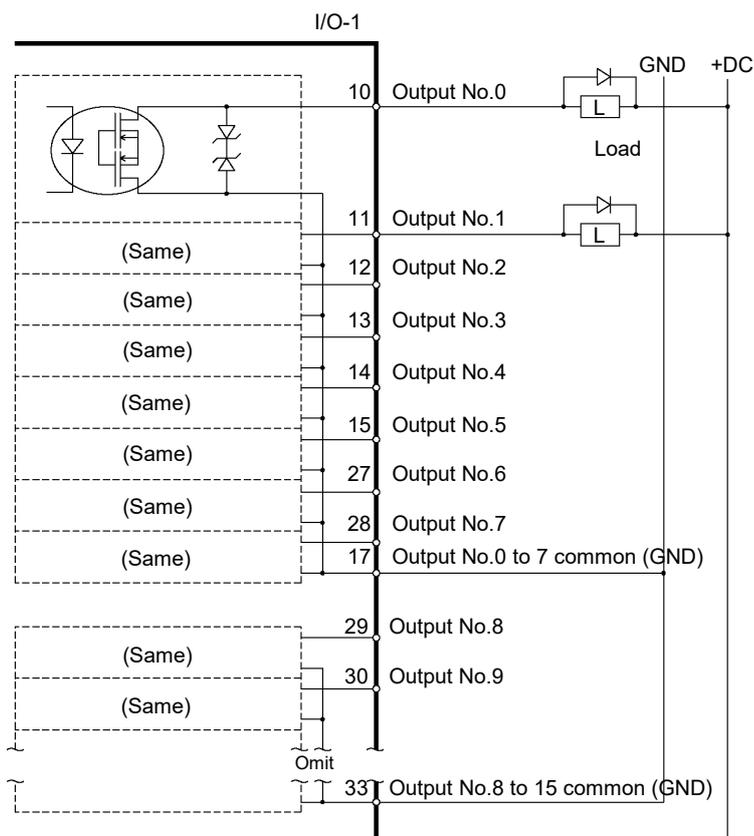
Typical Output Circuit Application 2: Source Type
