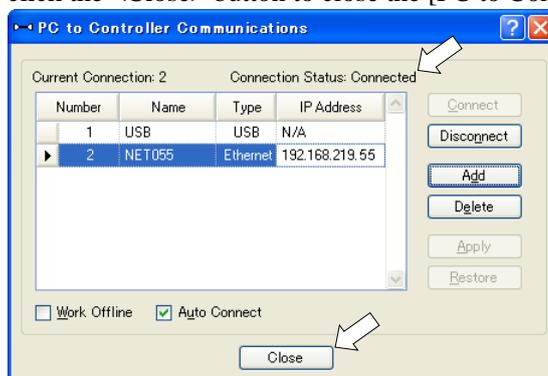
Connection between the development PC and the Controller is complete. Now the robot system can be used via an Ethernet connection from EPSON RC+ 7.0.
