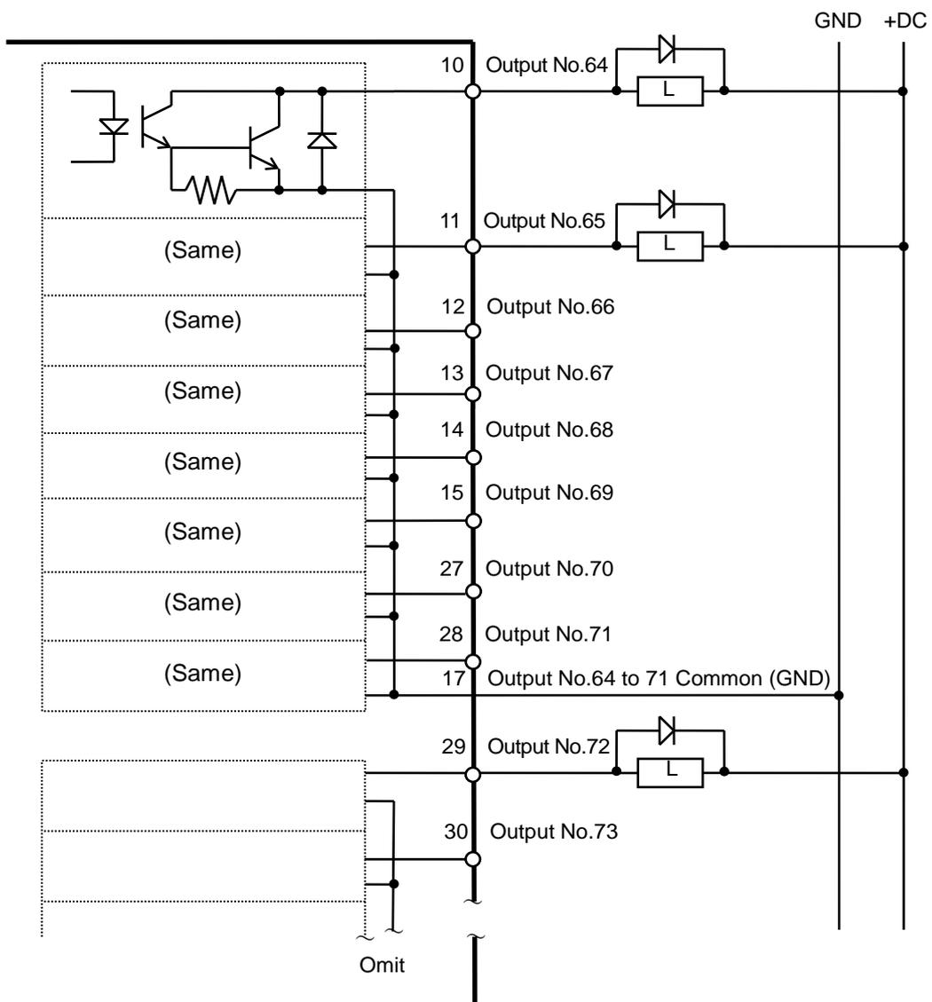
Typical Output Circuit Application 2: Source Type
