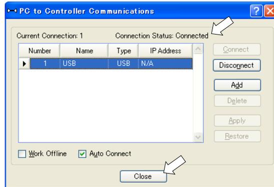
The connection between the development PC and the Controller is completed. Now the robot system can be used from EPSON RC+ 7.0.
