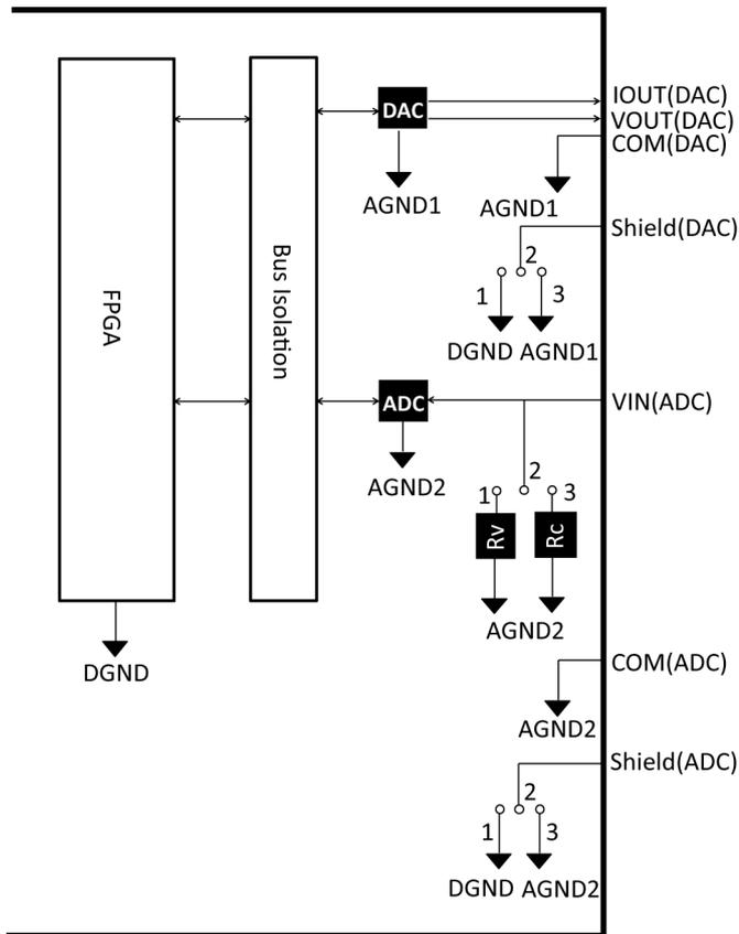
Rv: Voltage Input Terminating Resistance (100kΩ),
