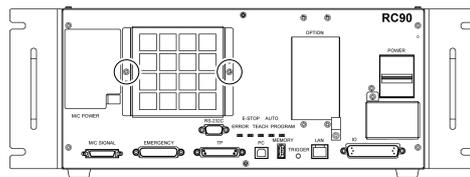
Vacuum off the dust when cleaning the filter.
