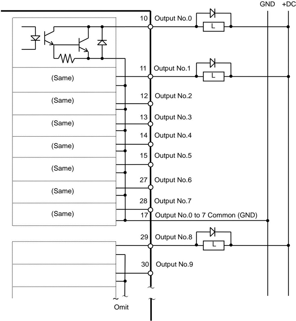
Typical Output Circuit Application 2: Source Type
