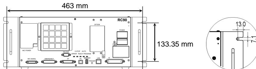
Ensure the draft around the in/out and prevent the other equipments, walls and install the Controller by keeping the distance as follows for maintenance.
