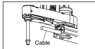
(22) Remove the spring plate mounting bolts on both the Arm #1 side and the Arm #2 side.
