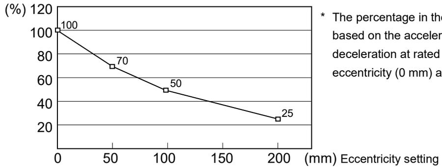
\* The percentage in the graph is based on the acceleration / deceleration at rated eccentricity (0 mm) as 100%.
