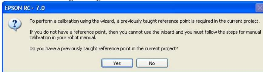
(3) Move the joint to calibrate manually to approximate 0 pulse position, as shown in the dialog. After moving the joint click the <Next> button.
