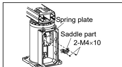
When using Wall mounting type
