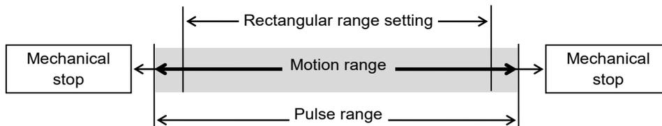
When the motion range is changed due to layout efficiency or safety, follow the descriptions in 5.1 to 5.3 to set the range.
