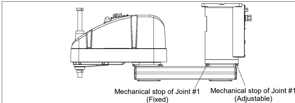
\* The different mechanical stop positions from Table Top mounting are indicated for Wall mounting and Ceiling mounting.
