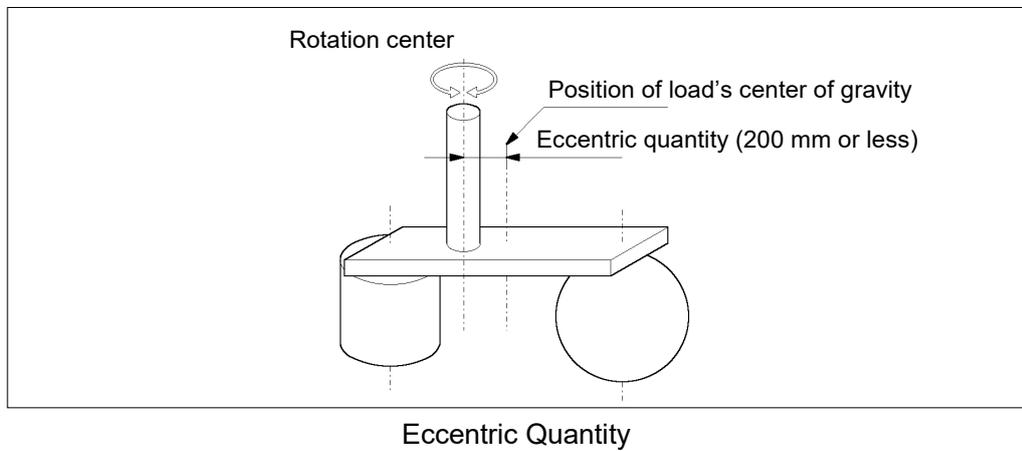
**Eccentric quantity of load on the shaft**
