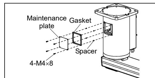
A gasket and spacers are installed to G10/G20-\*\*\*D\*, P\* (Protected-model).
