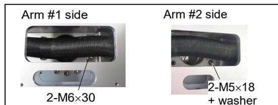
(23) Disconnect the cables to the base side.
