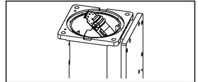
(6)-2 Mount the saddle part to mount the cables.
