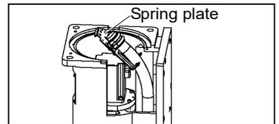
(6)-4 Move Arm #1 to the right or left until the arm touches the mechanical stop to make allowance.
