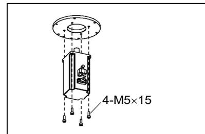
Joint #2 motor Installation
