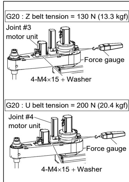
How to apply the proper tension to the U belt of G20
