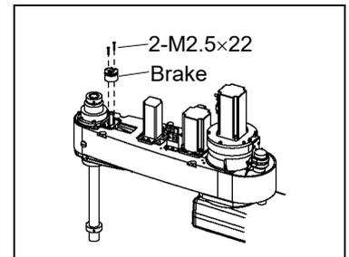
Joint #4 brake (1) Mount the brake.
