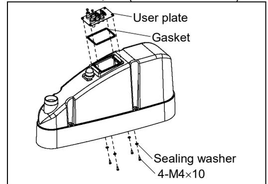
A gasket and sealing washers are installed to G10/G20-\*\*\*D\*, P\* (Protected-model).
