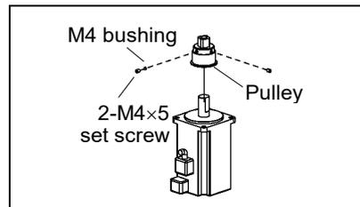
Joint #3 motor Installation
