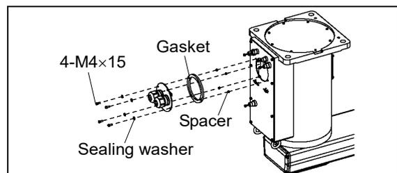
A gasket, spacers, and sealing washers are installed to G10/G20-\*\*\*D\*, P\* (Protected - model).
