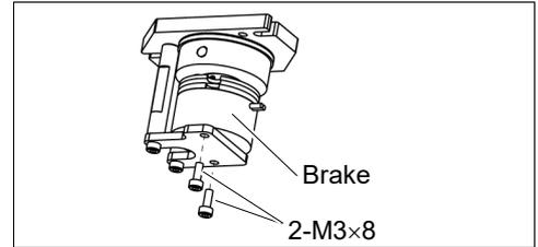
(2) Mount the brake hub to the pulley of the Joint #3 motor.
