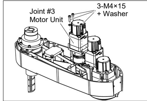
Apply the proper tension to the Z belt, and then secure the Joint #3 motor unit.
