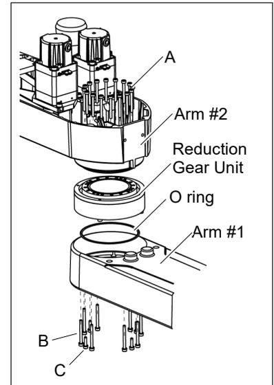
Loosely secure all bolts in a crisscross pattern so that the bolts will be secured evenly. Then, using a torque wrench, tighten each bolt securely in a crisscross pattern at the torque specified in the table below.
