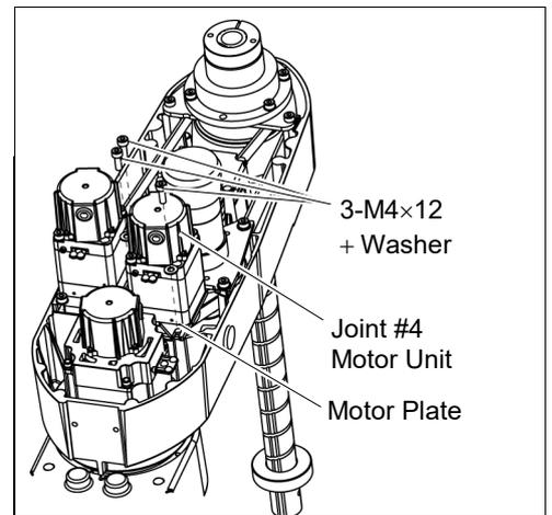
**NOTE** Make sure the motor unit can be moved by hand, and it will not tilt when pulled.
