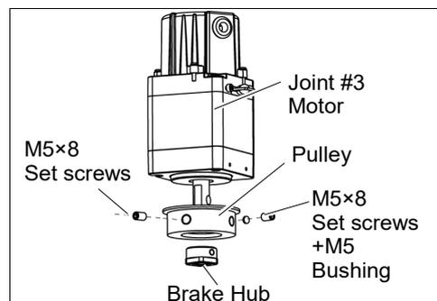
Joint #3 motor Installation (1) Mount the pulley and the brake hub to the Joint #3 motor.
