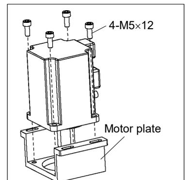
Joint #2 motor Installation
