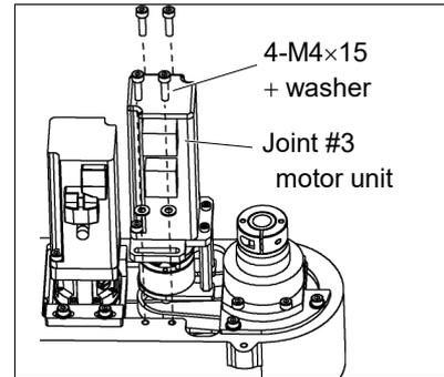
(10) Remove the Joint #3 motor unit from Arm #2.
