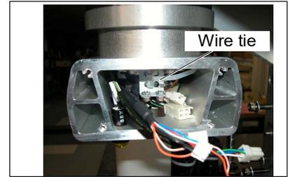
(22) Remove the Connector plate.
