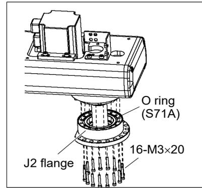
(17) Remove the reduction gear unit.
