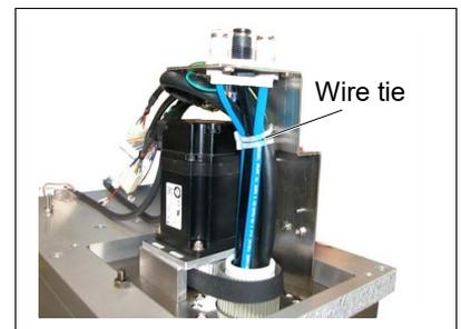
(26) Pull out the cable unit 2 and air tubes.
