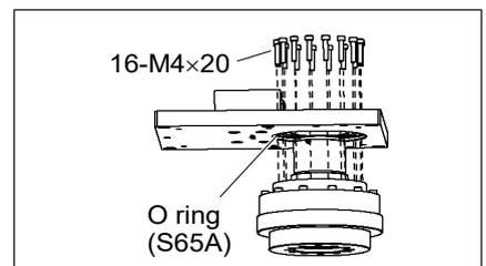
(10) Remove the J1 ring falling-off-prevention screws and remove the J1 ring.
