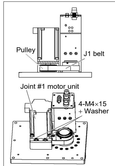
(4) Apply the proper tension to the J1 belt and secure the Joint #1 motor unit.
