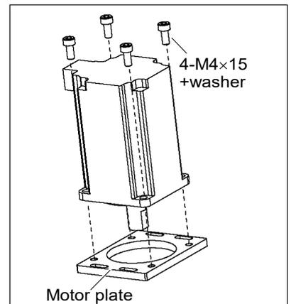
Joint #1 motor Installation (1) Mount the motor plate on the Joint #1 motor.
