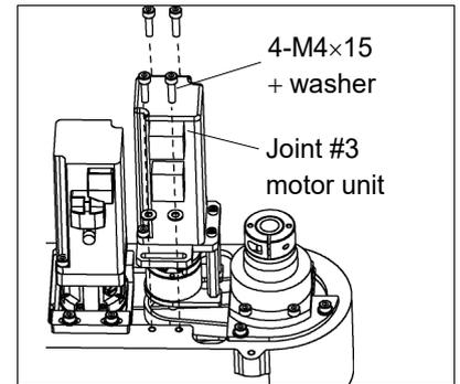
(11) Remove the Joint #3 motor unit from Arm #2.
