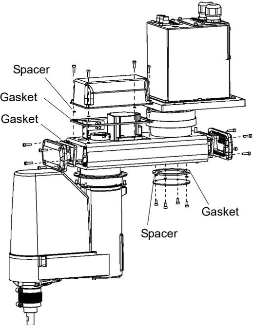
Gaskets and spacers are installed to Cleanroom-model.
