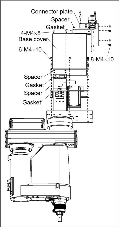
Gaskets and spacers are installed to the Cleanroom-model.
