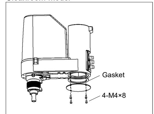
Gasket is installed to the Cleanroom-model.
