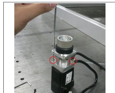
**Joint #4 Motor Installation**
