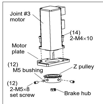
Joint #3 motor Installation
