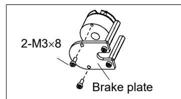
Electromagnetic Brake Installation
