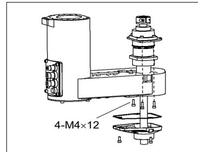
(17) Pull the ball screw spline unit out of Arm #2.
