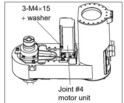
(13) Remove the Joint #4 motor unit from Arm #2.
