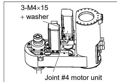
(12) Remove the Joint #4 motor unit from Arm #2.
