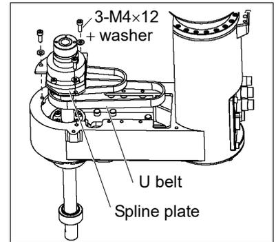
(2) Loosely secure the Spline plate to Arm #2.
