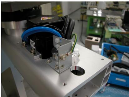
If the maintenance window is not designed in the base table, the Arm #1 cover cannot be removed. It needs to remove the Manipulator from the base table for the maintenance work. Be sure to remove the Manipulator from the base table by two or more personnel. For details, refer to *RS series Manual Environments and Installation*.
