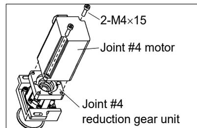
If the motor cannot be removed easily, put a washer between the motor and reduction gear and use the motor mounting screws to press the motor equally from the reduction gear side to remove the motor.
