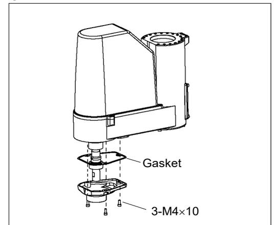
A gasket is installed to Cleanroom-model.
