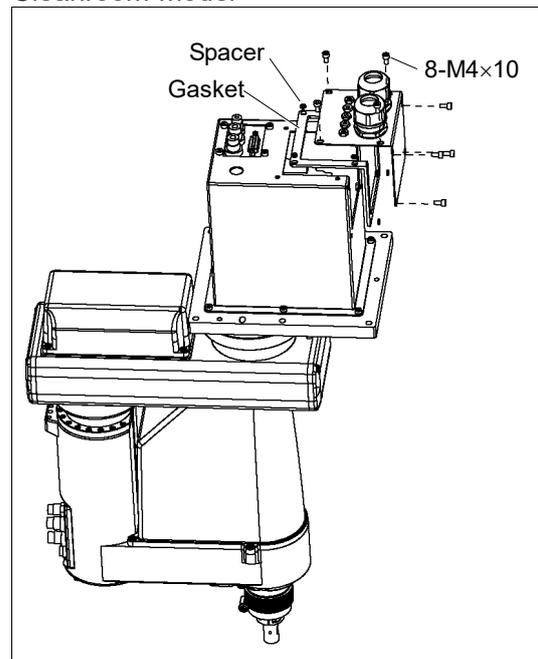
A gasket and spacer are installed to Cleanroom-model.
