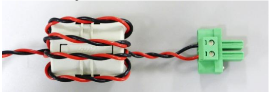
*Ferrite core: Kitagawa Industries Co., LTD RFC-20
