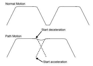
Two CP motions (Arc, Arc3, Go, Jump, Jump3, Jump3CP, Move), or two PTP motions (Go, Jump) compound the motion track by CP On.
