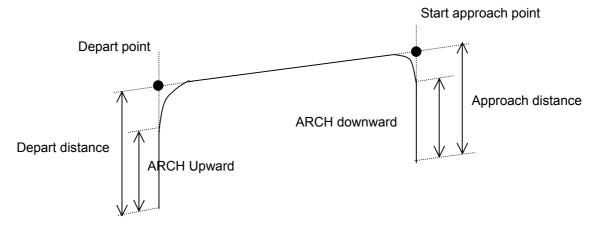
**Jump3CP** uses the SpeedS speed value and AccelS acceleration and deceleration values. Refer to *Using Jump3CP with CP* below on the relation between the speed/acceleration and the acceleration/deceleration. If, however, the ROT modifier parameter is used, **Jump3CP** uses the SpeedR speed value and AccelR acceleration and deceleration values. In this case SpeedS speed value and AccelS acceleration and deceleration value have no effect.
