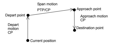
Arch motion is achieved by specifying the arch number. The arch motion for Jump3, Jump3CP is as shown in the figure below. For arch motion to occur, the Depart distance must be greater than the arch upward distance and the Approach distance must be greater than the arch downward distance.
